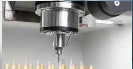
2 kW spindle and minimum-quantity coolant system
