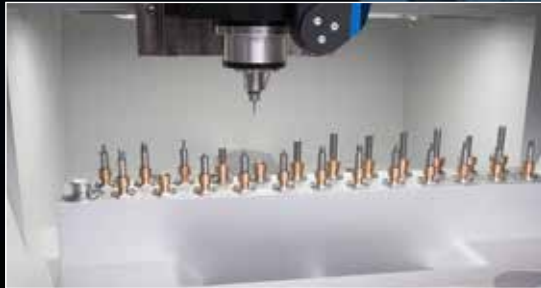
24-station tool magazine with integrated tool-length sensor
