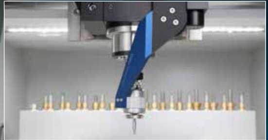
3D probe (XYZ sensor) and camera
